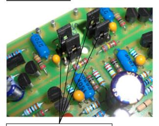
There are four Jumpers positioned on the phono board factory set to MM.
