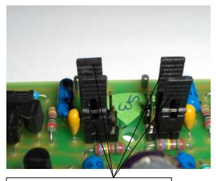
Moving the JUMPERS to the outer positions increases the gain for MC cartridges.
